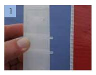
Insert the '4 x prongs' of the signAclip into the flutes of the flute board and push the clip all the way onto your sign.
